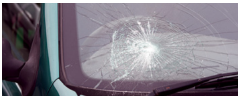
Chipped and cracked glass
