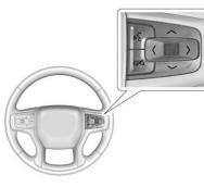
Use the right steering wheel control to open and scroll through the different items and displays.
