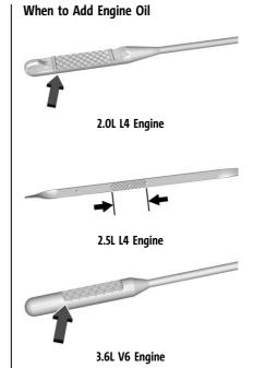
If the oil is below the cross-hatched area at the tip of the dipstick and the engine has been off for at least 15 minutes, add 1 L (1 qt) of the recommended oil and then
