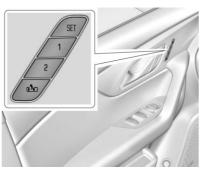
If equipped, memory seats allow two drivers to save and recall their unique seat positions for driving the vehicle, and a shared exit position for getting out of the vehicle. Other feature positions may also be saved, such as power mirrors and power steering wheel, if equipped. Memory positions are linked to RKE transmitter 1 or 2 for automatic memory recalls.
