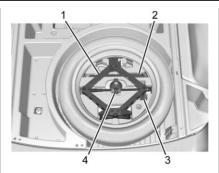
Turn the wing nut (4) counterclockwise to remove the jack (1), wheel wrench (2), and strap (3). Place the tool container near the tire being changed.
