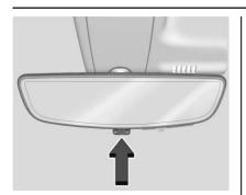
Pull the tab to turn on the display. Push the tab to turn it off. When off the mirror is automatic dimming. Adjust the mirror for a clear view of the area behind the vehicle while the display is off.
