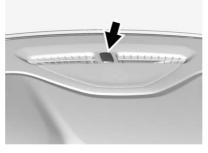
There is a light sensor on top of the instrument panel. Do not cover the sensor.
