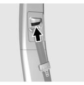
Press and hold the release button while raising or lowering the height adjuster to the desired position. After the height adjuster is set to the desired position, try to move it down without pressing the release button to make sure it has locked into position.
