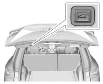
Press any liftgate button or the touch pad while the liftgate is moving to stop it. Pressing again restarts the operation in the reverse direction. The touch pad in the liftgate handle cannot be used to close the liftgate.
