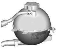
Check to see if coolant is visible in the coolant surge tank. If the coolant inside the coolant surge tank is boiling, do not do anything else until it cools down. See *Engine Overheating*  $\Rightarrow$  271.
