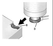
Slide the base of the tire sealant canister (3) into the slot on the top of the compressor (6) to hold it upright.
