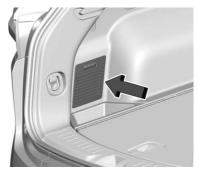
The rear compartment fuse block is behind a trim cover on the driver side of the rear storage compartment.
