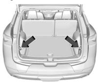
Two cargo tie-downs are located in the rear compartment of the vehicle. The tie-downs can be used to secure small loads.
