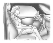
If a person of adult size is sitting in the front outboard passenger seat, but the OFF indicator is lit, it could be because that person is not sitting properly in the seat or that the child restraint locking feature is
