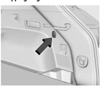
There is a shopping bag hook on each side of the rear cargo area. Press the hook to open. The maximum weight per hook is 5 kg (11 lb). **Cargo Tie-Downs**
