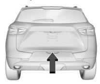
To open the liftgate, press the touch pad in the liftgate handle and lift up. Unlocking all doors will also unlock the liftgate.
