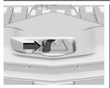
2. Go to the front of the vehicle and locate the secondary release lever under the front center of the hood. Push the secondary hood release lever to the right to release.  After you have partially lifted the hood, the gas strut system will automatically lift the hood and hold it in the fully open position.
