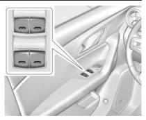
The power windows work when the ignition is on, in ACC/ACCESSORY, or when Retained Accessory Power (RAP) is active. See Retained Accessory Power (RAP)  $\Rightarrow$  205.
