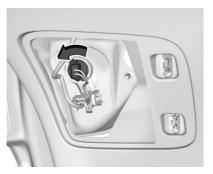
Turn the bulb socket counterclockwise and pull the bulb straight out of the socket. 4. Replace the bulb and reverse Steps 1–3 to reinstall.
