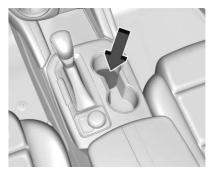
3. Place the new transmitter into the front cupholder.
