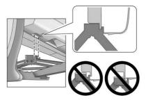
Turn the wheel wrench clockwise to raise the jack until the slot in the jack lift head fits into the metal flange located behind the cut out on the plastic molding.
