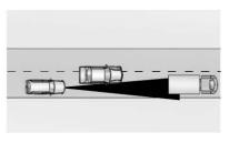
ACC will not detect a vehicle ahead until it is completely in the lane. The brakes may need to be manually applied.
