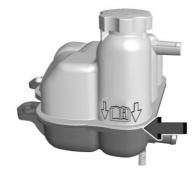
If coolant is visible but the coolant level is not at or above the indicated mark, add a 50/50 mixture of clean drinkable water and DEX-COOL coolant.
