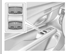
Power windows work when the ignition is on, in ACC/ACCESSORY, or when Retained Accessory Power (RAP) is active. See *Retained Accessory Power (RAP)* ⇒ 223.
