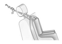
If the position you are using has an adjustable head restraint and you are using a dual tether, raise the head restraint and route the tether under the head restraint and in between the head restraint posts.
