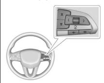
Press  $\leq$  or  $\geq$  to access the cluster applications. Use the thumbwheel to scroll  $\wedge$  or  $\vee$  through the list of available features. Press the thumbwheel to select. Not all applications will be available on all vehicles.
