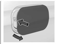
To open the fuel door, push and release the rearward center edge of the door.
