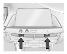
Adjustable air vents are in the center and on the sides of the instrument panel, and on the rear of the center console storage. Move the slider knobs to change the direction of or to close off the airflow.
