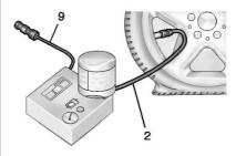
Attach the sealant/air hose (2) to the tire valve stem by turning it clockwise until tight. 8. Plug the power plug (9) into the accessory power outlet in the vehicle. Unplug all items from other accessory power outlets. See *Power Outlets* ♀ 85.
