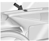
The light sensor is on top of the instrument panel or on the windshield near the rearview mirror. Do not cover the sensor, otherwise the headlamps will come on when they are not needed.
