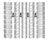
Treadwear indicators are one way to tell when it is time for new tires. Treadwear indicators appear when the tires have only 1.6 mm (1/16 in) or less of tread remaining. See *Tire Inspection*  $\Rightarrow$  352 and *Tire Rotation*  $\Rightarrow$  352 for additional information.
