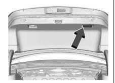
Close the trunk by pulling on the handle. Do not use the handle as a tie-down. Do not press the touch pad while closing the trunk; this will cause the trunk lid to be unlatched.
