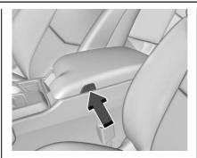
Press the button and lift to access the storage area. There is an accessory power outlet, two USB ports, and an SD card slot inside. See *Power Outlets*  $\Rightarrow$  85 or USB Port  $\Rightarrow$  145
