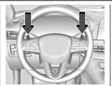
If equipped, vehicles with Tap Shift have controls on the back of the steering wheel to manually shift the automatic transmission.
