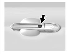
When the doors are locked and the remote key is within 1 m (3 ft) of the driver door handle, press the lock/ unlock button. When unlocking from the driver door, the first press unlocks that door; press again within five seconds to unlock the passenger door and the trunk. See *Remote Keyless Entry (RKE) System Operation* ⇔ 7.
