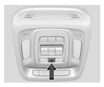
It is recommended that the intrusion and inclination sensor be deactivated if pets are left in the vehicle or the vehicle is being transported. With the vehicle turned off, press in the front overhead console. The indicator light will come on momentarily, indicating that these sensors have been disabled for the next alarm system arming cycle.
