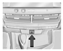
\(\triangle : Press this button to make the front and rear turn signal lamps flash on and off. Release the button for at least one second and press again to turn the flashers off.
