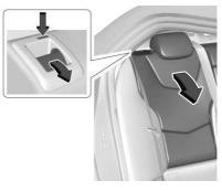
Pull the lever on top of the seatback toward you to unlock the seatback.
