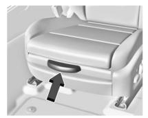
If equipped, pull up on the lever. Then pull or push on the support to lengthen or shorten. Release the lever to lock in place.
