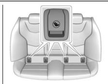
The lower anchors are located under the labeled covers on the seat cushion near the crease between the seatback and the seat cushion.
