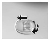
1. Slide lamp to the front and remove it out of the front wing with the rear end.
