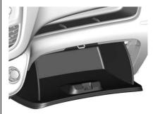
Inside the glovebox there is a compartment for the Owner's Manual. Pull the lug to open the compartment. The glovebox should be closed whilst driving.
