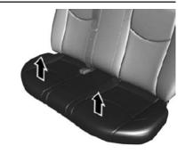
2. Pull up on the front edge of the rear seat cushion to release it.
