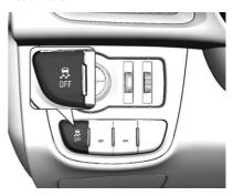
For very high-performance driving ESC can be deactivated: Hold & depressed for approx. 5 seconds.
