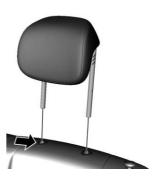
Press the catch, pull the head restraint upwards and remove.
