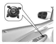
Select the relevant exterior mirror by turning the control to left (L) or right (R). Then swivel the control to adjust the mirror. In position 0 no mirror is selected.
