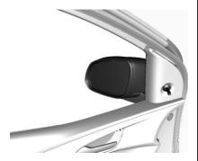
If equipped, move the control up, down, or side to side to adjust the mirror.
