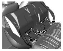
To remove the rear seat cushion, push the hinges in direction of arrow.
