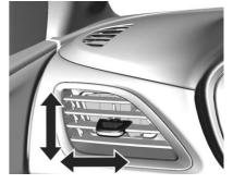
Direct the flow air by tilting the slats.
