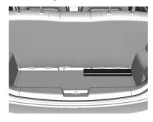
Stow the warning triangle in the space on the load compartment.
