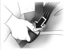
To release belt, press red button on belt buckle.
