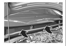
The air intake in front of the windscreen in the engine compartment must be kept clear to allow air intake. Remove any leaves, dirt or snow.
