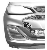
Screw in the towing eye as far as it will go until it stops in a horizontal position. (Should be contact with tow nut.)
