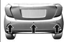
The rear parking assist makes parking easier by measuring the distance between the vehicle and rear obstacles. It informs and warns the driver by giving acoustic signals and display indication.
