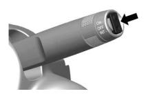
Press the rocker switch to activate the rear window wiper:
