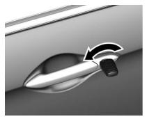
Manually unlock the driver's door by turning the key in the lock. Switch on the ignition and press the central locking button to unlock all doors, load compartment.
