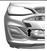
Disengage cap by using the screwdriver and remove the cap.
