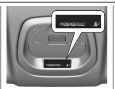
♣2 for front passenger seat illuminates or flashes red in the overhead console when the seat is occupied.
