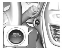
Electronic key must be inside the vehicle.
