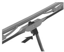
Lift wiper arm. Press release lever and detach wiper blade.
