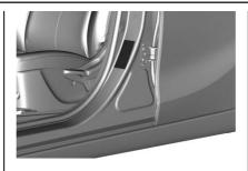
The tire pressure information label on the left door frame indicates the original equipment tires and the correspondent tire pressures.
