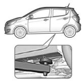
Rear arm position of the lifting platform located centrally under the recess of the sill.
