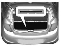
Stow the warning triangle in the vehicle tool box below the floor cover in the load compartment.
