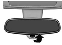
To reduce dazzle, adjust the lever on the underside of the mirror housing.
