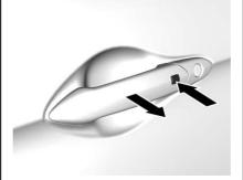
Electronic key system: Unlocking the vehicle by pressing the button on any exterior door handle deactivates antitheft alarm system.
