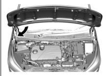
Lift the hood and release the hood prop rod from the prop rod retainer, which is under the hood.
