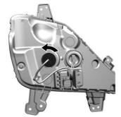
2. Remove the turn signal lamp or Type 1 DRL bulb rotating anticlockwise.
