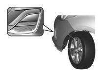
1. Turn the front wheels and remove 2 push nuts on outside of wheel liner.
