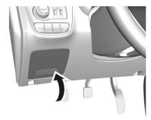
In left-hand drive vehicles, the fuse box is behind the storage compartment in the instrument panel.
