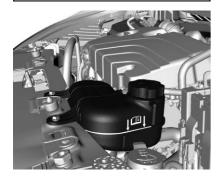
If the cooling system is cold, the coolant level should be above the filling line mark.
