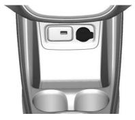
A 12 Volt power outlet is located in the center console.
