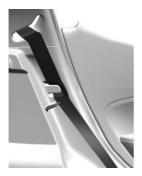
5. Put the seat belts for the outboard seats into the belt guides.
