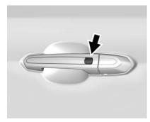
If equipped, use the Keyless Access system to lock and unlock the door. When the doors are locked and the RKE transmitter is within 1 m (3 ft) of the driver door handle, press the lock/unlock button. When unlocking from the driver door, the first press unlocks that door; press again within five seconds to unlock all passenger
