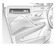
The rear door safety locks prevent passengers from opening the rear doors from inside the vehicle. Press a to activate the safety locks on the rear doors. The indicator light in the switch will illuminate when activated.
