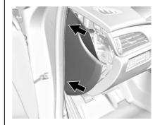
To install the end cover, insert the tabs on the back of the cover into the slots in the instrument panel at the points shown. Align the clips with the slots in the instrument panel, and press the cover into place.
