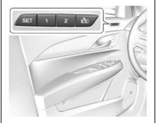
If equipped, memory seats allow two drivers to store and recall their unique seat positions for driving the vehicle, and a shared exit position for getting out of the vehicle. Other feature positions may also be set, such as power mirrors and power steering wheel, if equipped. Memory positions are linked to RKE transmitter 1 or 2 for automatic memory recalls.
