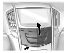
If equipped with storage behind the climate control system, touch the bottom of the climate control panel until the door starts to open. Touch the bottom of the climate control panel again until the door automatically starts to close.
