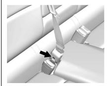
Disconnect the rear seat belt mini-latch using a key in the slot on the mini-buckle, and let the belt retract.
