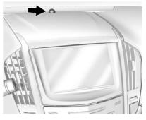
The solar sensor monitors the solar heat.
