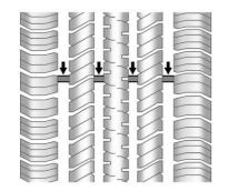
Treadwear indicators are one way to tell when it is time for new tires. Treadwear indicators appear when the tires have only 1.6 mm (1/16 in) or
