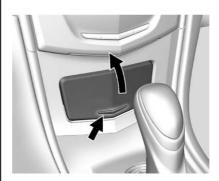
To access, press on the cover and release. There is an accessory power outlet inside. See *Power Outlets* ⇔ 112.
