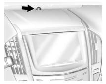
The solar sensor monitors the solar heat
