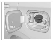
The fuel cap is behind a hinged fuel door on the driver side of the vehicle. To open the fuel door, push and release the rearward center edge of the door.
