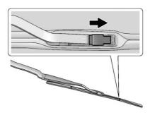
Lift up on the latch in the middle of the wiper blade where the wiper arm attaches.
