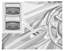
The power windows work when the ignition is on, in ACC/ACCESSORY, or when Retained Accessory Power (RAP) is active.
