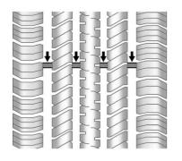
Treadwear indicators are one way to tell when it is time for new tires. Treadwear indicators appear when the tires have only 1.6 mm (1/16 in) or less of tread remaining. See *Tire Inspection*  $\Rightarrow$  313 and *Tire Rotation*  $\Rightarrow$  314.
