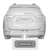
To open the liftgate, press the touch pad on the bottom of the liftgate and lift up.
