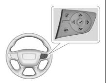
Press  $\triangleleft$  or  $\triangleright$  to select VEHICLE menu, then use  $\triangle$  or  $\nabla$  to scroll through the menu items to select TCS/StabiliTrak.
