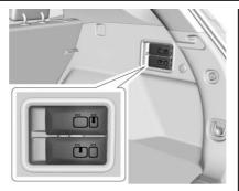
If equipped, the rear seatbacks can also be folded forward by pulling the levers on the passenger side of the rear cargo area.
