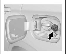
DEF is a non-toxic solution that is sprayed into the exhaust stream of diesel vehicles to cause a chemical reaction and break down NOx emissions into harmless nitrogen and water.
