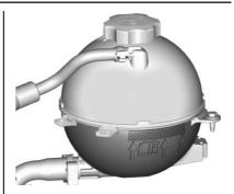
Check to see if coolant is visible in the coolant surge tank. If the coolant inside the coolant surge tank is boiling, do not do anything else until it cools down. If coolant is visible but the coolant level mark is not visible, add a 50/50 mixture of clean, drinkable water and DEX-COOL coolant at the coolant surge tank to the top rib on the middle of the tank, but be sure the cooling system is cool before this is done. See *Engine Overheating* \$\times 280.
