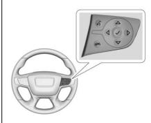
Press  $\triangleleft$  to access the cluster applications. Use  $\triangle$  or  $\nabla$  to scroll through the list of available applications.
