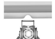
Locate the notch on the sheet metal weld flange. Place the center of the jack lift head on the center of the sheet metal notch.
