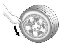
Turn the wheel wrench counterclockwise to loosen all the wheel nuts, but do not remove them yet.
