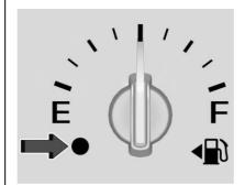
For the base level cluster, this light comes on when the fuel tank is low on fuel. The light turns off when fuel is added. If it does not, have the vehicle serviced.
