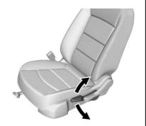
Move the lever up or down to manually raise or lower the seat.
