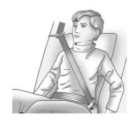
Buckle, position, and release the seat belt as described previously in this section. Make sure the shoulder belt crosses the shoulder. The belt should be close to, but not contacting, the neck.
