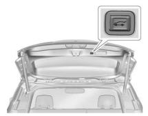
Press on the bottom of the liftgate next to the pull cup to close.
