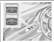
The power windows work when the ignition is on, in ACC/ACCESSORY, or in Retained Accessory Power (RAP). See Retained Accessory Power (RAP) ⇒ 192.
