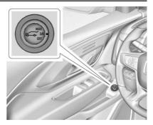
If equipped with a power liftgate, the switch is usually on the driver door. The switch can also be on the overhead console. The vehicle must be in P (Park).
