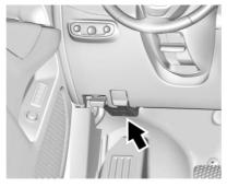
The instrument panel fuse block is under the instrument panel on the driver side.
