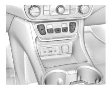
The shift switches are on the front shift console. The selected gear position will illuminate red on the shift switch, while all others will be displayed in white. If the shift is not immediate, as in very cold conditions, the indicator on the shift switch may blink until it is fully engaged.
