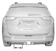
To operate, kick your foot straight up in one swift motion under the rear bumper between the left exhaust pipe and the license plate, then pull it back.
