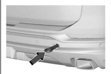
Install the tow eye into the socket by turning it until it stops.
