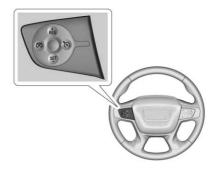
: Press to turn the cruise control system on and off. A white indicator comes on in the instrument cluster when cruise control is turned on.
