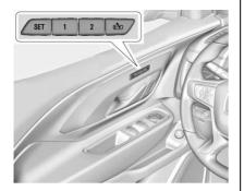
If equipped, memory seats allow two drivers to store and recall their unique seat positions for driving the vehicle, and a shared exit position for getting out of the vehicle. Other feature positions may also be set, such as power mirrors, if equipped. Memory positions are linked to RKE transmitter 1 or 2 for automatic memory recalls.
