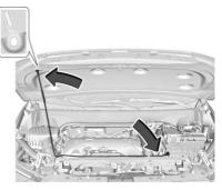
Release the hood prop from its retainer, located above the radiator. Securely place the hood prop into the slot on the underside of the hood.
