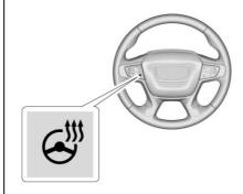
: If equipped, press to turn it on or off. A light next to the button displays when the feature is turned on. The steering wheel takes about three minutes to start heating.
