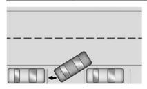
APA will instruct the vehicle to stop once a large enough space is found. Follow the displayed instructions. When instructed to drive in reverse, shift to R (Reverse) to engage automatic steering. The steering wheel will briefly vibrate as a reminder to remove hands from the steering wheel. Check surroundings and continue braking or accelerating as needed, and be prepared to stop to avoid vehicles, pedestrians, or objects.
