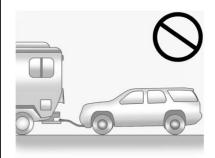
The vehicle was not designed to be towed with all four wheels on the ground. The vehicle may be towed
