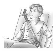
Buckle, position, and release the safety belt as described previously in this section. Make sure the shoulder belt crosses the shoulder. The belt should be close to, but not contacting, the neck.
