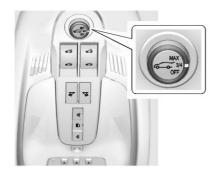
If equipped, the power liftgate switch is on the overhead console. The vehicle must be in P (Park) to operate. The taillamps flash when the power liftgate moves.
