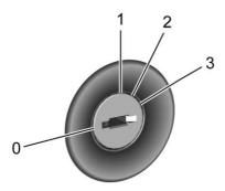
The ignition switch has four different positions.
