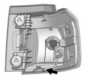
11. Verify that the taillamp assembly tab, located at the bottom of the taillamp assembly, is aligned to the fascia bracket before securing with screws.
