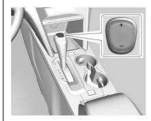
**P**: This position locks the front wheels. Use P (Park) when starting the engine because the vehicle cannot move easily.
