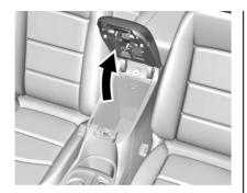
There is an accessory power outlet inside. There may also be a USB port and an auxiliary input jack inside.
