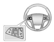
To turn LDW on and off, press the LANE DEPART button on the steering wheel. The control indicator will light when LDW is on.
