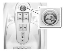
On vehicles with a power liftgate, the vehicle must be in P (Park) to use the power feature. The taillamps flash when the power liftgate moves. Choose the power liftgate mode by turning the dial on the switch to either the 3/4 or MAX position.
