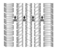
Treadwear indicators are one way to tell when it is time for new tires. Treadwear indicators appear when the tires have only 1.6 mm (1/16 in) or less of tread remaining. See *Tire Inspection* ⇒ 247 and *Tire Rotation* ⇒ 247.
