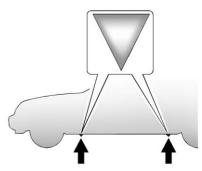
4. Position the jack lift head at the jack location nearest the flat tire. The location is indicated by a mark on the bottom edge of the front and rear door plastic molding. The jack must not be used in any other position.
