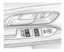
Press the front of the switch to open the window. Pull the switch up to close it.
