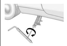
Raise the vehicle by turning the jack handle clockwise. Raise the vehicle far enough off the ground so there is enough room for the road tire to clear the ground.
