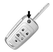
Press the button on the RKE transmitter to extend the key. Press the button and the key blade to retract the key.
