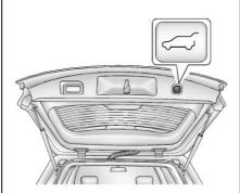
Press and release  $\leftarrow$  on the liftgate next to the latch to close the liftgate.
