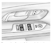
Press the front of the switch to lower the window. Pull the switch up to raise it.
