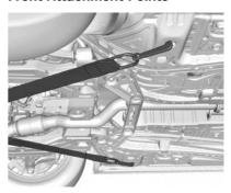
The vehicle is equipped with specific attachment points to be used by the towing provider. These holes may be
