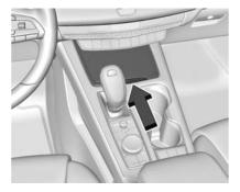
To open the front storage compartment, slide the cover forward. There are two USB ports inside. To close, push the cover forward and let go.
