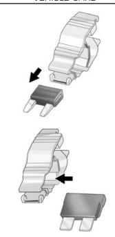
Use the fuse puller to remove the fuse from the top or side, as shown above.
