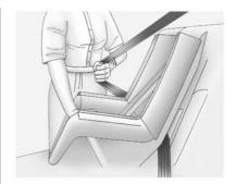
5. Pull the shoulder belt all the way out of the retractor to set the lock. When the retractor lock is set, the belt can be tightened but not pulled out of the retractor.
