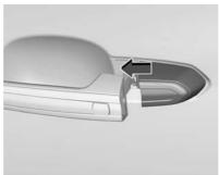
Slide the cap forward and press the forward edge to install the cap in place.
