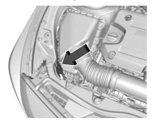
Open the hood and unwrap the electrical cord. The cord is located on the passenger side of the compartment near the air cleaner/ filter.
