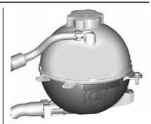
Check to see if coolant is visible in the coolant surge tank. If the coolant inside the coolant surge tank is boiling, do not do anything else until it cools down. If coolant is visible but the coolant level mark is not at or above the indicated mark, add a 50/50 mixture of clean, drinkable water and DEX-COOL coolant. Be sure the cooling system is cool before this is done. See *Engine Overheating* ⇔ 296.
