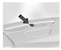
The solar sensor, on top of the instrument panel near the windshield, monitors the solar intensity.
