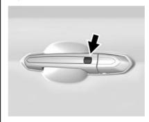
The RKE transmitter must be within 1 m (3 ft) of the door or liftgate being opened. Press the button on the door handle to open. See "Keyless Access" in *Remote Keyless Entry (RKE) System Operation* ⇔ 7.
