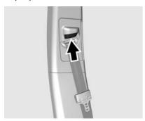
Press and hold the release button while raising or lowering the height adjuster to the desired position. After the height adjuster is set to the desired position, try to move it down without pressing the release button to make sure it has locked into position.
