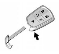
To remove the key, press the button near the bottom of the transmitter, and pull the key out. Never pull the key out without pressing the button.
