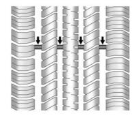
Treadwear indicators are one way to tell when it is time for new tires. Treadwear indicators appear when the tires have only 1.6 mm (1/16 in) or less of tread remaining. See *Tire Inspection*  $\Rightarrow$  329 and *Tire Rotation*  $\Rightarrow$  330 for additional information.
