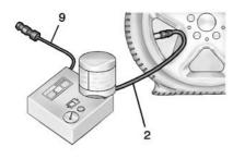
Attach the sealant/air hose (2) to the tire valve stem by turning it clockwise until tight. 8. Plug the power plug (9) into the accessory power outlet in the vehicle. Unplug all items from other accessory power outlets. See *Power Outlets* ⇔ 96.
