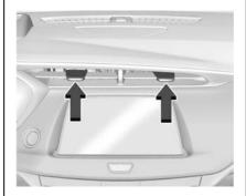
Adjustable air vents are in the center and on the sides of the instrument panel, and on the rear of the center console storage.
