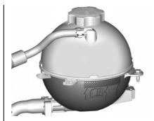
3. If topping off the level in the coolant surge tank, add the proper mixture until the level reaches the mark on the front of the tank and replace the cap. Operate the vehicle. Repeat steps 1–3, as necessary.
