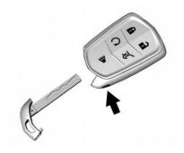
Press the button on the side of the RKE transmitter near the bottom and pull the key out. Never pull the key out without pressing the button.
