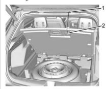
Insert the hook (2) into the opening on the liftgate (1) to hold it open.
