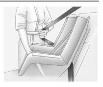
4. Pull the shoulder belt all the way out of the retractor to set the lock. When the retractor lock is set, the belt can be tightened but not pulled out of the retractor.
