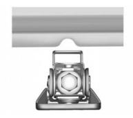
Locate the notch on the sheet metal weld flange. Place the center of the jack lift head on the center of the sheet metal notch.
