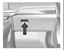
Lift the handle to open the glove box. Close until it latches. Use the vehicle key to lock or unlock. See  $Keys \Leftrightarrow 6$ .
