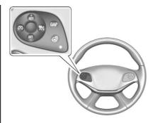
ৰ্ম্জ: Press to turn the system on or off. A white Adaptive Cruise Control indicator comes on.
