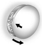
The fuel cap is behind the fuel door on the passenger side of the vehicle. To open the fuel door, push and release the rearward center edge of the door.
