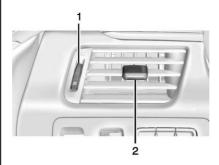
Move the thumbwheels (1) up or down to open or close off the airflow.
