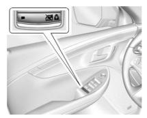
Press to activate the safety locks on the rear doors. The indicator light in the switch will illuminate when activated.
