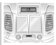
If equipped with storage behind the radio, press ☐ and hold to open. There is a USB port inside. See USB Port ⇒ 165.
