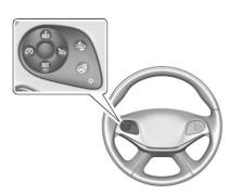
: Press to turn cruise control on or off. A white indicator comes on in the instrument cluster when cruise is on.
