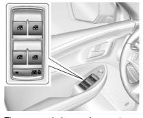
The power windows only operate with the ignition in ACC/ ACCESSORY or ON/RUN/START. or when Retained Accessory Power (RAP) is active. See Retained
