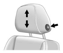
To raise or lower the head restraint, press the button located on the side of the head restraint, and pull up or push the head restraint down and release the button. Pull and push on the head restraint after the button is released to make sure it is locked in place.
