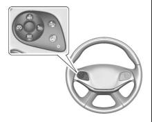
: Press to turn cruise control on or off. A white indicator comes on in the instrument cluster when cruise is on.
