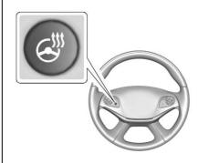
If equipped, press to turn on or off. A light on the button displays when the feature is turned on.
