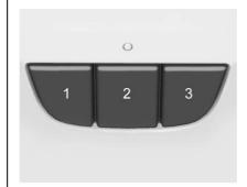
This system provides a way to replace up to three remote control transmitters used to activate devices such as garage door openers, security systems, and home automation devices.
