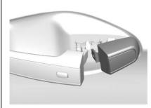
Insert the two tabs (7) at the back of the cap (8) between the seal (5) and the metal base (6).
