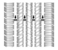
Treadwear indicators are one way to tell when it is time for new tires. Treadwear indicators appear when the tires have only 1.6 mm (1/16 in) or less of tread remaining. See *Tire Inspection*  $\Rightarrow$  297 and *Tire Rotation*  $\Rightarrow$  297.
