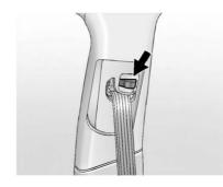
Push down on the release button and move the height adjuster to the desired position. The adjuster can be moved up by pushing the slider/ trim up. After the adjuster is set to the desired position, try to move it down without pushing the release button to make sure it has locked into position.
