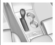
**P**: This position locks the front wheels. It is the best position to use when you start the engine because the vehicle cannot move easily.
